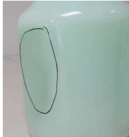
**Panel sink 2** The panels on this bottle have begun to sink, but have not yet affected the adhesion of the label.
