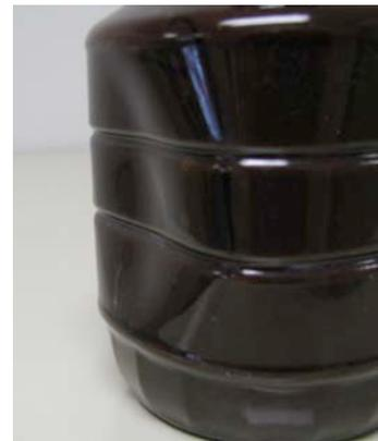
**Panel sink 3** The design of this bottle did not provide enough strength to resist panel sink.
